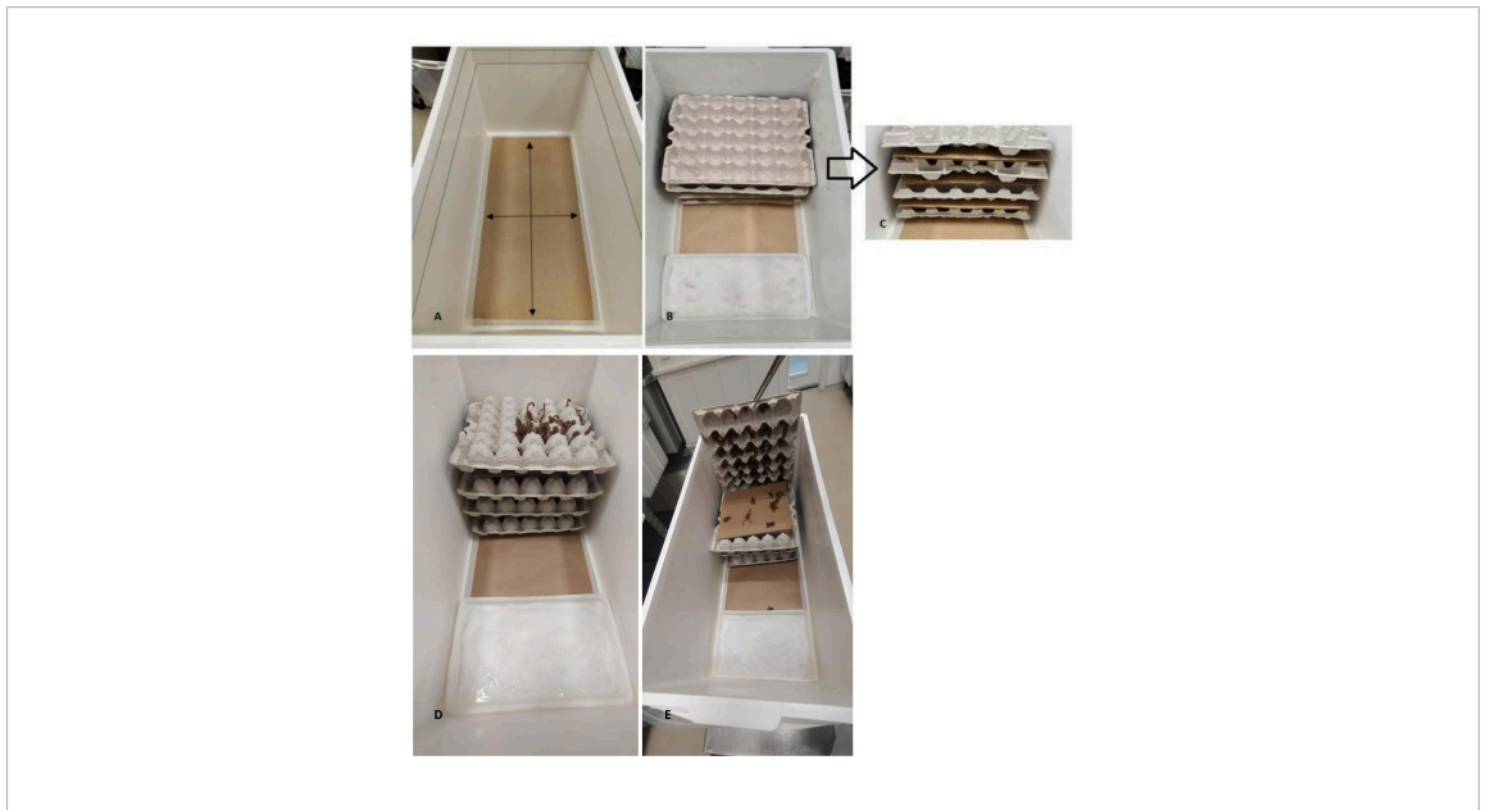
Figure 3: Housing and enclosure preparation. (A) Arrows indicate the kraft paper on the bottom, fixed with masking tape on the edges. Dotted lines indicate the self-adhesive plastic tape placed on the top of the internal surface of the enclosure. (B) Vertical substrate (egg trays piled on one side of the container) and a shallow polypropylene tray (water tray) placed on the opposite side. (C) Vertical substrate detail: egg trays piled with a rigid cardboard sheet in between two trays. (D) Cardboard sheets and egg trays positioned in layers, simulating the natural dark and humid habitat of T. serrulatus . (E) Animals accommodated in the substrate. Please click here to view a larger version of this figure.
